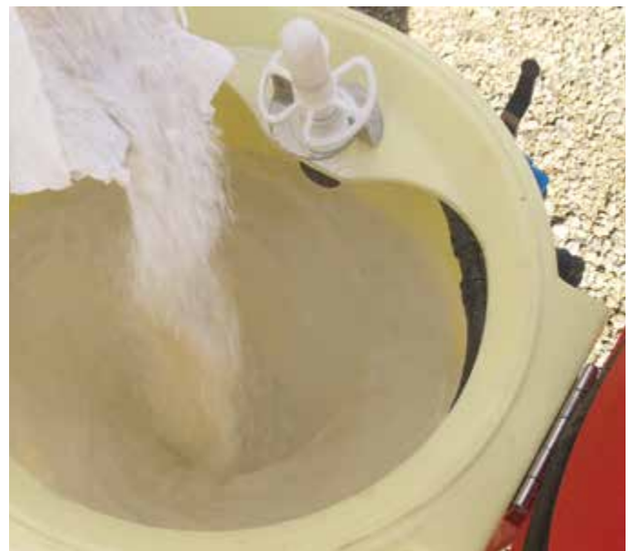
Pre-mixing Surround in the water vortex of a Grani-pot is quick and effective.
